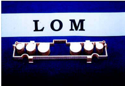
Figure 8.4: Benchmark test piece made from Laminated Object Manufacturing (LOM)
