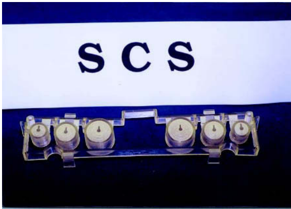
Figure 8.6: Benchmark test piece made from Solid Creation Systems (SCS)
