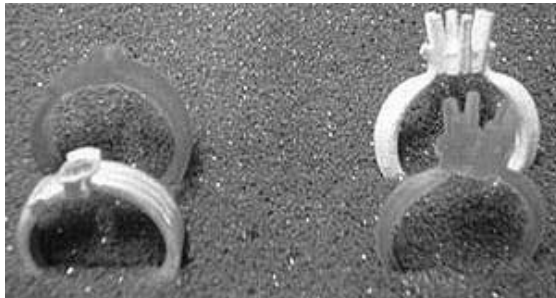
Figure 3.27: Resin ring models and metal casted ring models (Courtesy Meiko Co. Ltd.)
