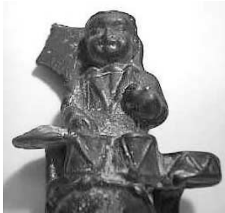
Figure 3.42: Metal model made by investment casting with ice pattern
