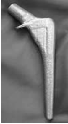
Figure 5.16: Medical LENS produced metal part (Courtesy of Optomec Inc.)
