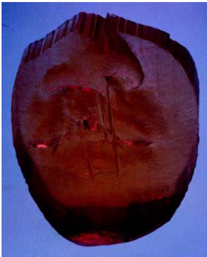
Figure 7.13: SLA model of a patient's facial details
