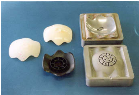
Figure 3.16: RP model (left), the ABS injection molding (center) and the low cost metal die (right) (Courtesy Teijin Seiki Co. Ltd.)
