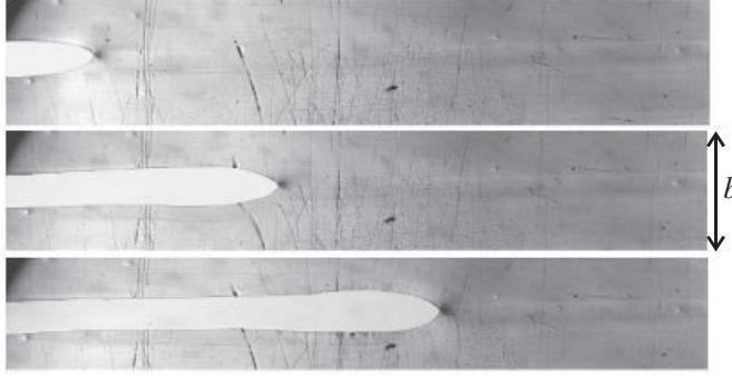
Figure 13.4 Time evolution of a crack in a finite strip of soft polyacrylamide gel. Note the transition from an effectively infinite medium accompanied by a change of the tip shape when the crack length l \sim b . Reproduced from [113] with permission from the American Physical Society.
