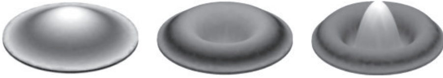
Figure 7.6 Shapes of the first three modes of vibration of a circular plate.
