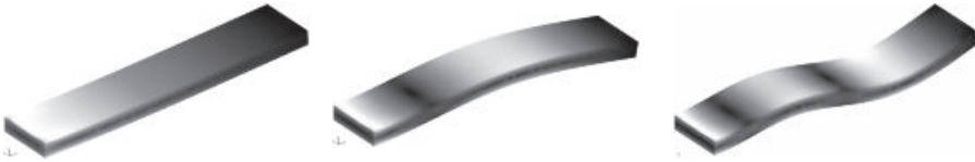
Figure 7.3 Mode shapes for the first three modes of vibration of a cantilever beam (the clamped end is the one on the left).
