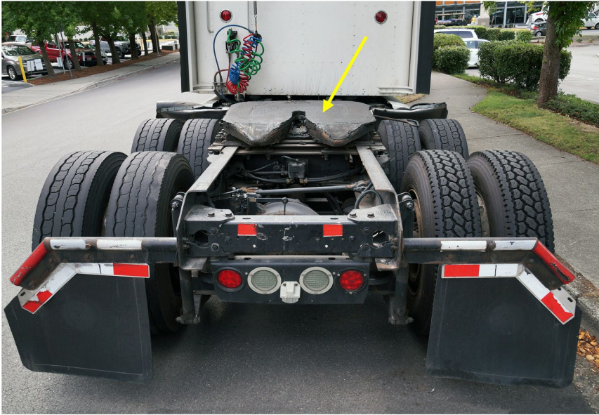
FIGURE 21 Rear view of a truck tractor showing the fifth wheel assembly.
