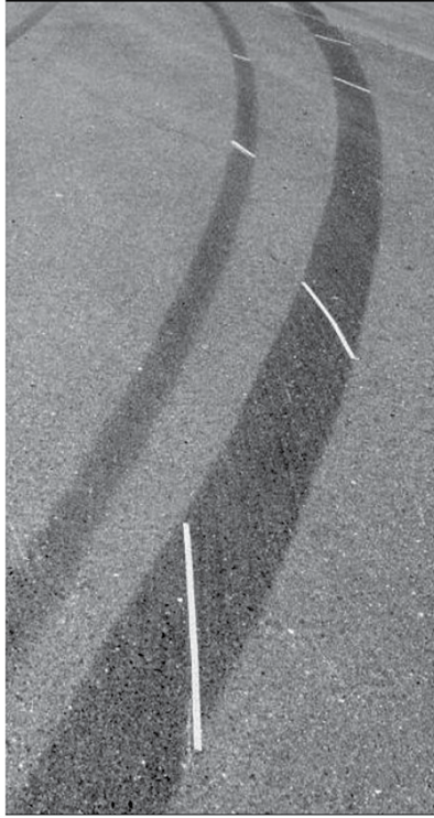
FIGURE 39 Striations in a tire mark (SAE 2009-01-0092).
