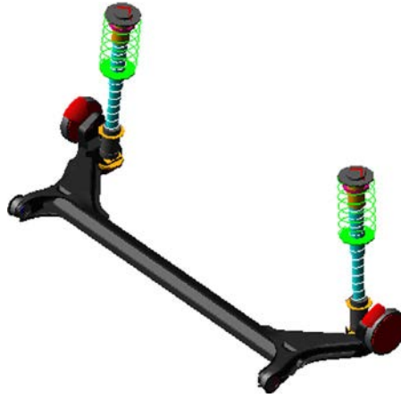
Fig. 2.4 Rear suspension set of the SEDAN vehicle.
