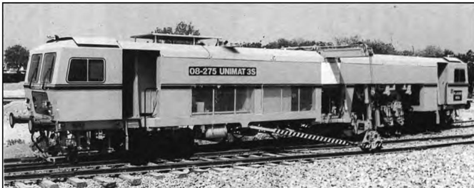
**Fig. 12.11 (b)** Unimat 08-275 3S switches and crossing tamping machine
