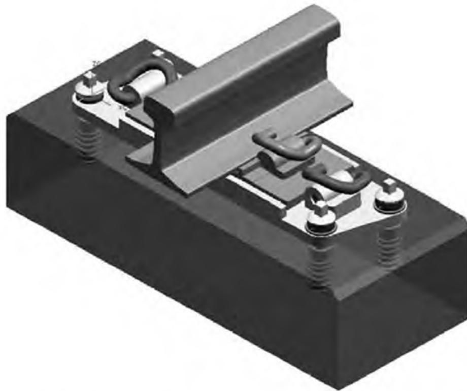
**Fig. 21.12** Plinth type ballastless track assemblies for main lines (See also Color Plate 20)
