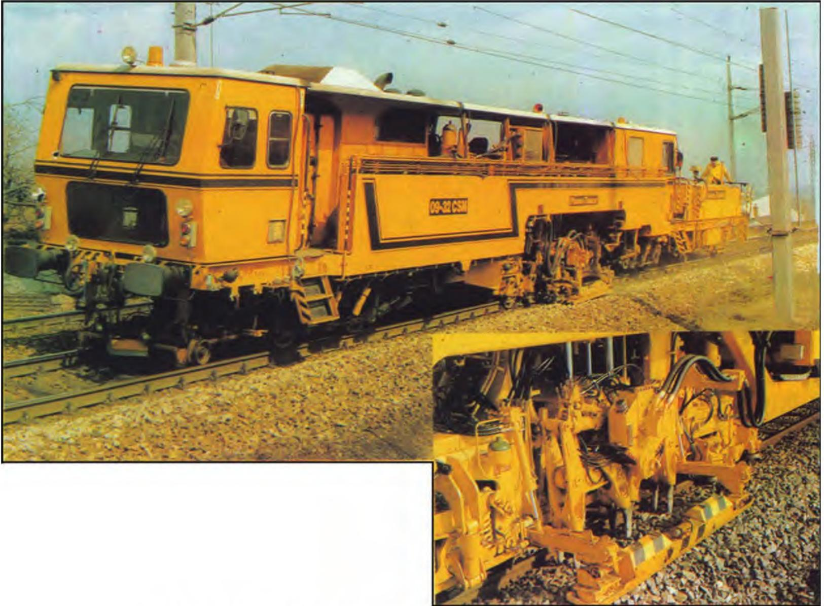
Fig. 12.13 09-CSM continuous action tamping machine
