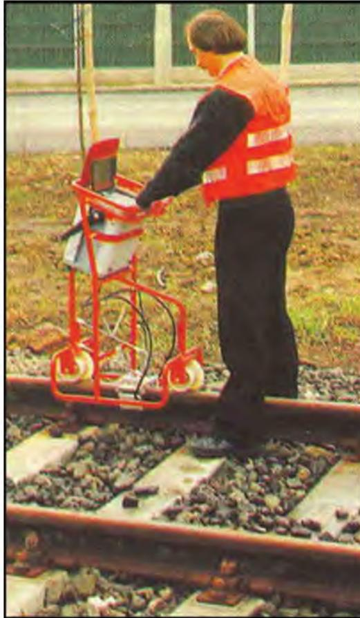
**Fig. 10.15** The rail scan equipment
