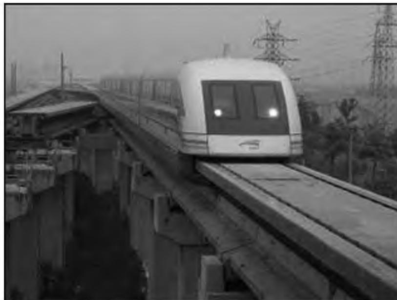
**Fig. 18.12** Transrapid magnetic levitation train in Shanghai (See also Color Plate 18)
