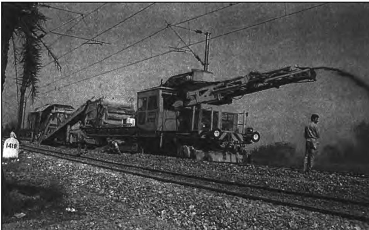
**Fig. 12.12** Ballast cleaning machine
