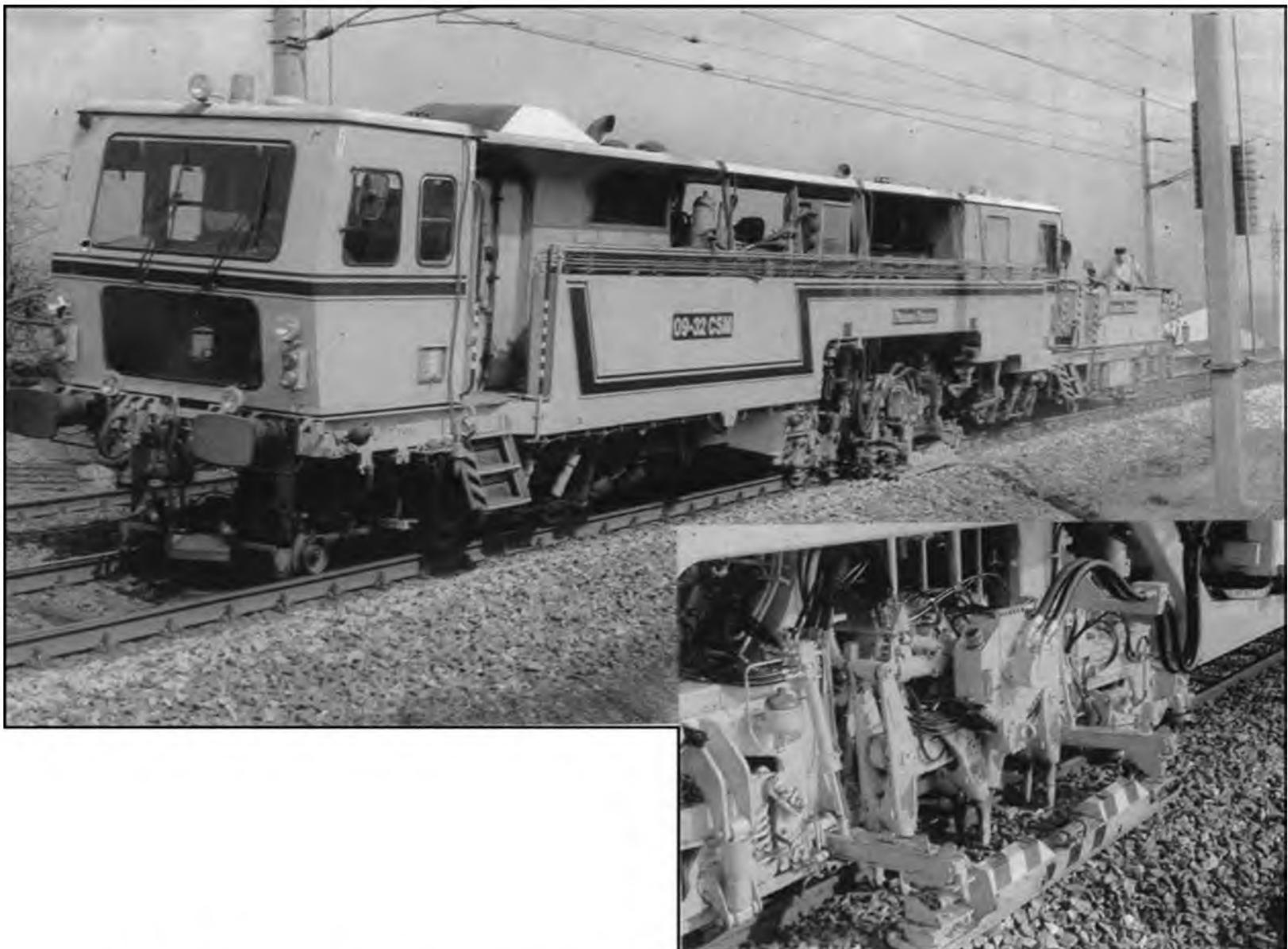
**Fig. 12.13** 09-CSM continuous action tamping machine (See also Color Plate 6)
