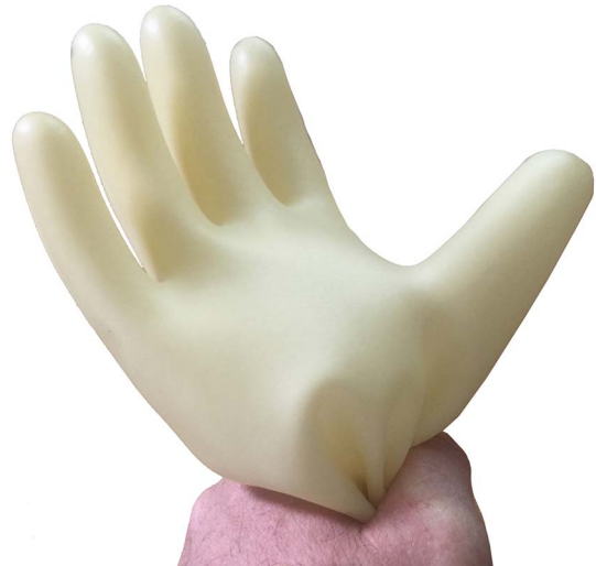
Figure 2.8 Electrical glove inflation test to check for cuts and damage
