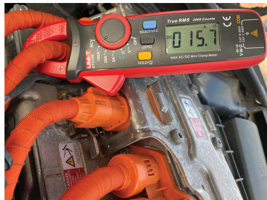
Figure 9.43 Clamp-type ammeter reading the current taken by the car heater
