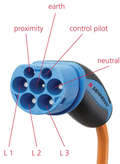
Figure 9.47 Connector has seven pins if three-phase and five if only single phase: Proximity (PP), Protective earth (PE), Control pilot (CP), Line 1 single phase (L1) and neutral (N), Lines L1, L2, L3 and neutral are used for three phase (Source: Mennekes)
