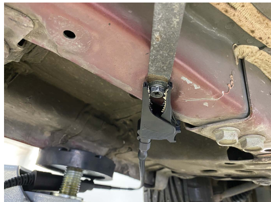
Figure 9.27 One option for connection that was NOT used (There are 4 of these bonding straps on the battery pack)
