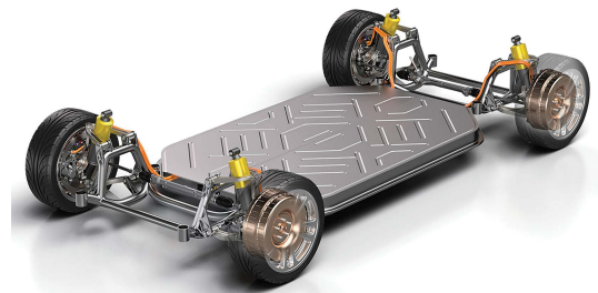
Figure 4.13 Mounting the motors in the wheels makes more space available for batteries, passengers or cargo (Source: Protean Electric)
