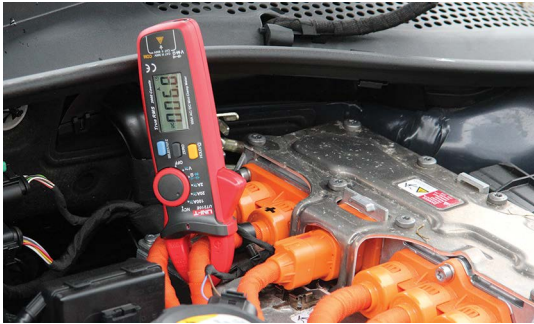
Figure 2.32 Inductive ammeter clamp on a high-voltage cable (measuring the current drawn by the EV cabin heater)
