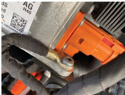
Figure 9.20 This bonding strap connects the case of a high-voltage component to the chassis on a Volkswagen Golf GTE
