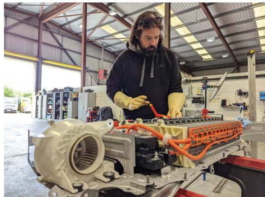
Figure 10.9 Battery pack work carried out in a well-ventilated workshop
