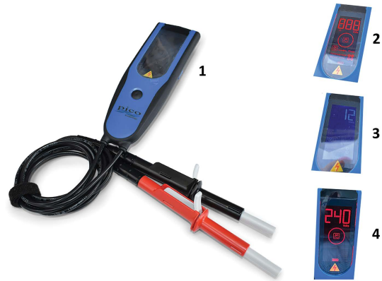
Figure 9.33 Two-pole tester and the four possible results (part of the PicoScope EV kit)
