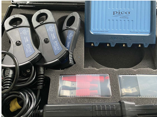
Figure 9.37 Top of the range PicoScope kit specially designed for EV diagnostics – note the three current clamps that can be used on each phase of the motor/generator circuit
