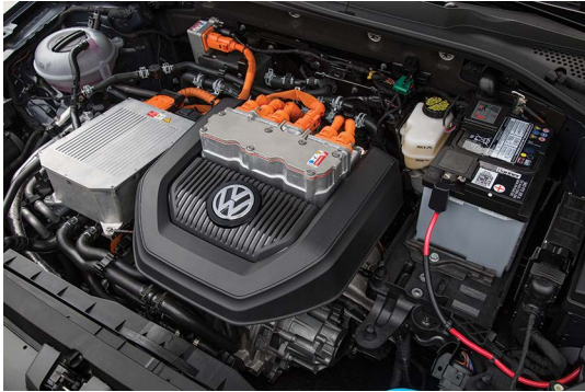
Figure 2.5 High-voltage cables are always orange (Source: Volkswagen Media)
