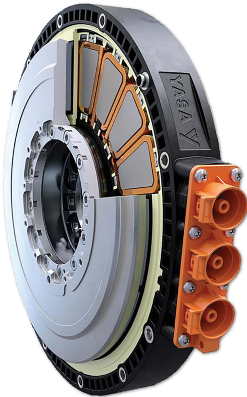
Figure 6.18 YASA axial electric motor, 260 Nm/180 kW 10 s peak, 65 mm length, 260 mm diameter, 12 kg, 15 W/kg (Source: YASA)
