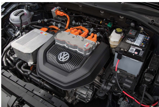
Figure 4.43 VW Golf-e showing some of the orange cables
