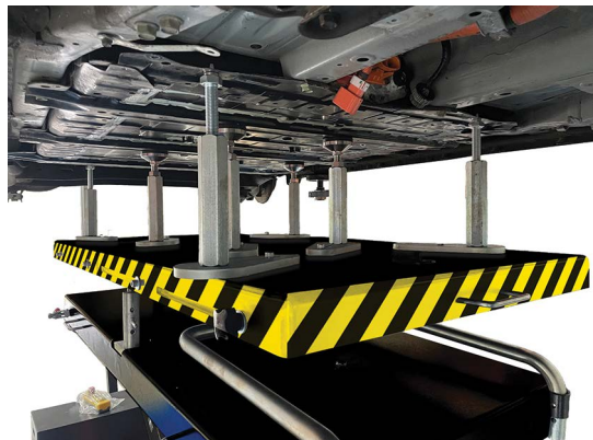
Figure 2.20 Battery lift in use with adaptors (Source: Snap-on/Sun Electric)
