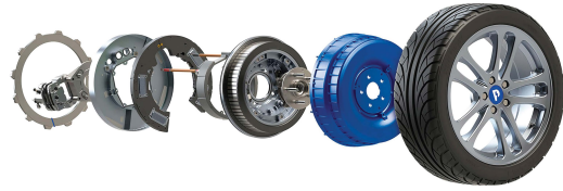
Figure 4.14 Protean Electric's in-wheel motor system is arguably simpler than a conventional electric automobile, which has constant-velocity joints, drive shafts and a centrally mounted transmission and motor (Source: Protean Electric)
