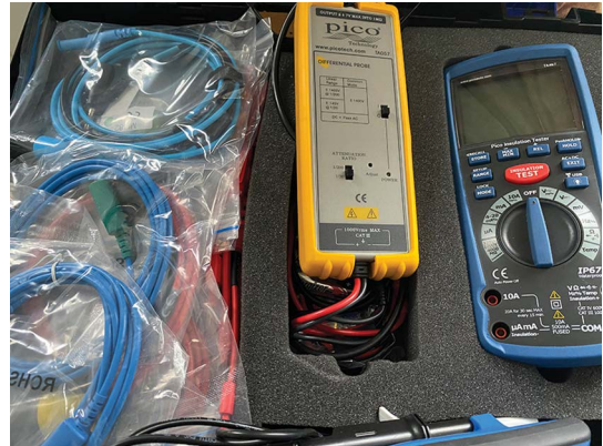
Figure 2.26 Electric vehicle PicoScope kit, cables, multimeter, and differential probe
