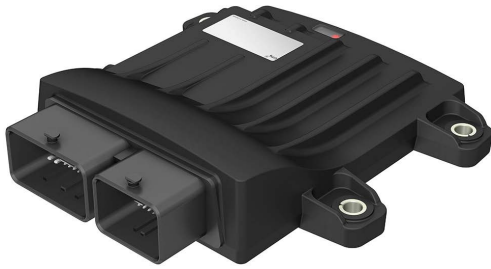
Figure 4.70 The appropriately named 'neuro 200' vehicle management unit is the brain of the system (Source: Dana)
