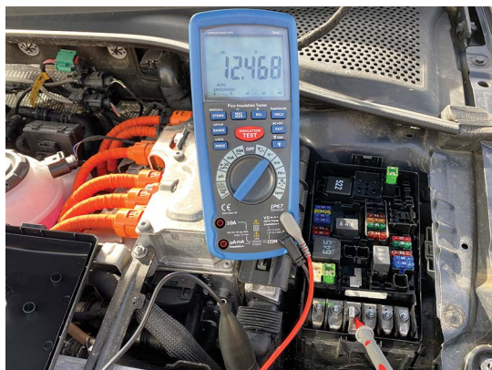
Figure 2.28 CAT IV meter in use (on low-voltage)
