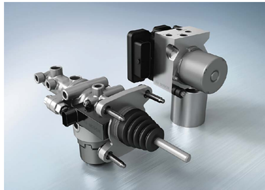
Figure 4.54 Vacuum-independent braking system specially designed for plug-in hybrids and electric vehicles. It comprises a brake operation unit (left) and an actuation control module (right), which supplement the ESP® hydraulic modulator (Source: Bosch Media)
