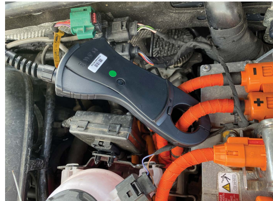
Figure 9.44 One of the three amp clamps supplied in the PicoScope EV kit connected around the high-voltage battery supply cable at the inverter
