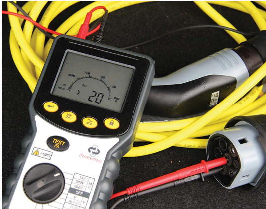
Figure 2.34 Checking insulation resistance between conductors in an EV charging lead (in this case the reading is >20 GΩ)
