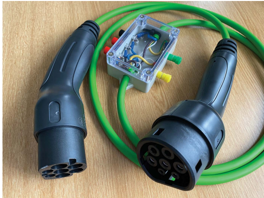
Figure 9.48 Homemade breakout box (green PE, yellow CP, black N, red L1 vehicle, red L1 EVSE to allow ammeter connection)
