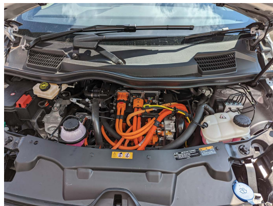
Figure 10.18 Mercedes EV with separate water-cooled systems for the AC system and HV battery pack
