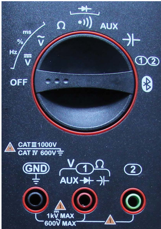
Figure 2.29 CAT III 1000 V and CAT IV 600 V meter
