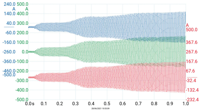
Figure 9.52 Accelerating from rest (frequency is about 120 Hz)
