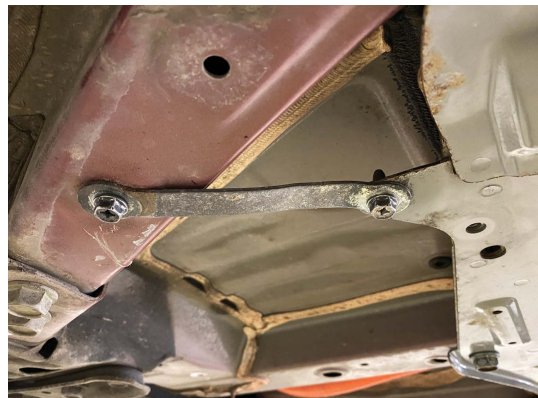
Figure 9.21 A bonding strap between the battery box and chassis on a Nissan LEAF
