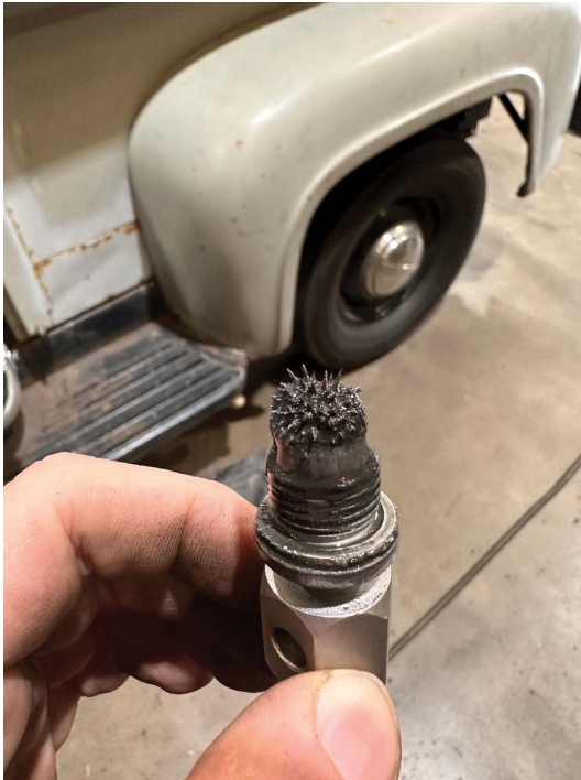
Figure 10.5 A drain plug from a failed single-speed box on a BMW i3, mileage 30,000 miles
