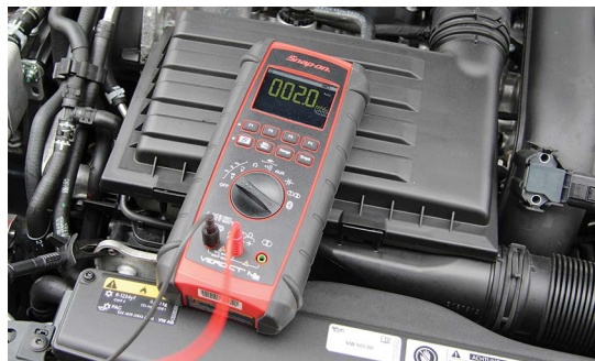
Figure 2.33 Ghost voltage caused by shaking the red lead
