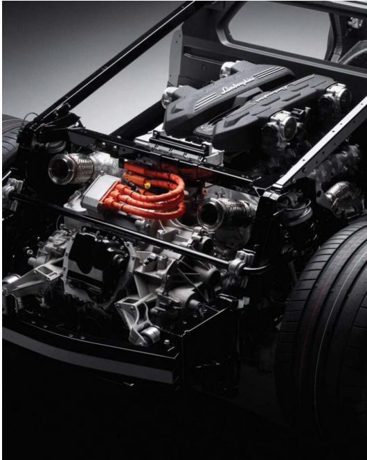
Figure 4.39 V12 engine and front drive motors (Source: Lamborghini Media)
