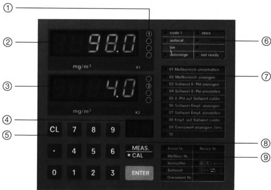
Fig. 6.17: Control panel of an NDIR gas analyzer with 2 measuring channels (Ultramat 5 E, Siemens AG)
