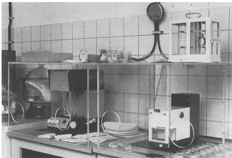
Fig. 7.26: View of a laboratory unit for conditioning and weighing of particle filters
