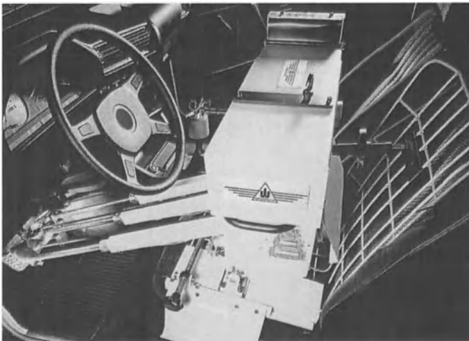
Fig. 8.12: Automatic driver installed in a vehicle (WECO and VW)
