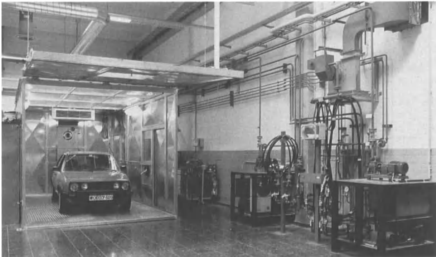
Fig. 8.35: View of an open SHED chamber
