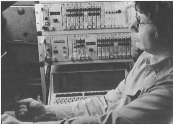
Fig 8.24: View of a torque measurement instrumentation mounted into a vehicle
