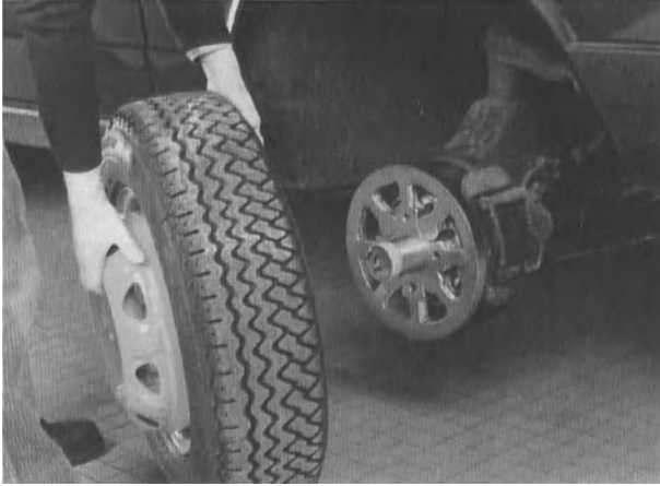
Fig. 8.23: View of a mounted torque sensor
