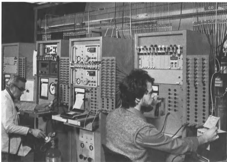
Fig. 8.32: View of the measuring instruments to check span gases
