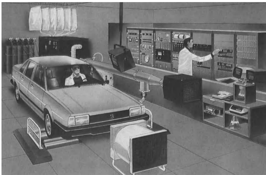
Fig 8.1: Phantom drawing of an exhaust emission laboratory
